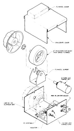
fig. 1. Construction of the varactor tuned master frequency oscillator. Brass flywheel provides very smooth tuning from one end of a band to the other.
